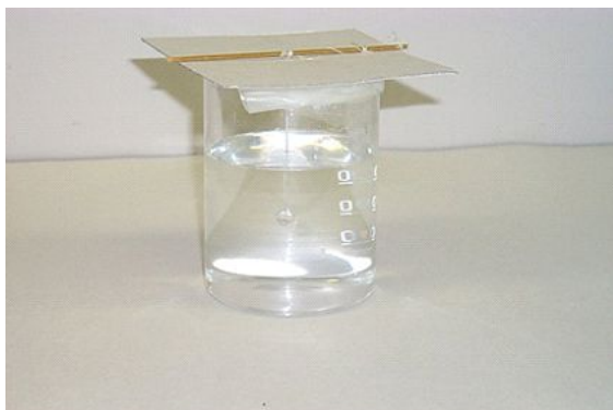
Figure 2. Seed crystal of alum suspended in saturated solution. (Credit: picture by Luc Van Meervelt)
